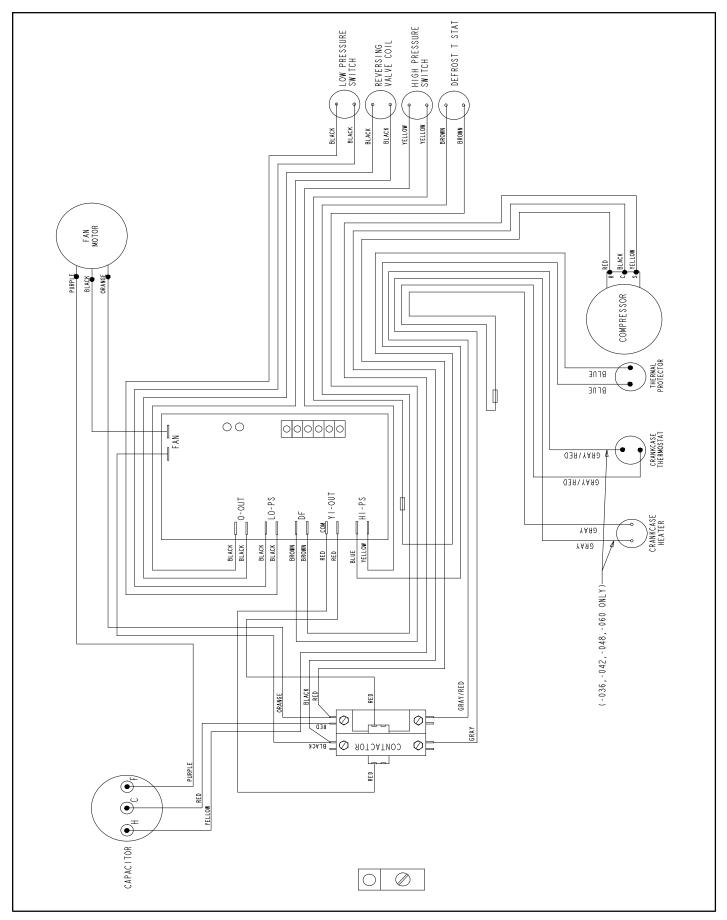
Figure 17. Typical Factory Wiring (Interlink Compressor)
